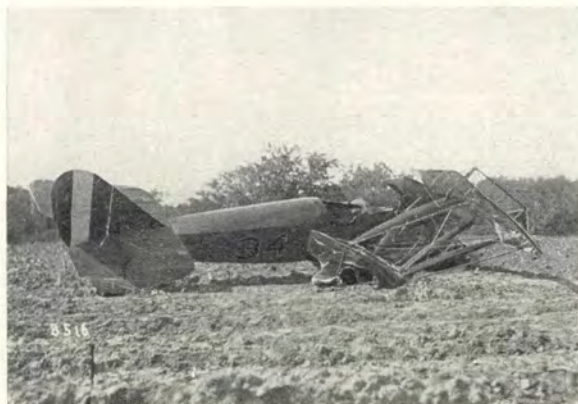
Pilot of this JN4-1 flew into heavy fog, lost his bearings because of inadequate "blind flight" training and equipment, and in attempting to spiral down struck the trees at the edge of the field and crashed.
